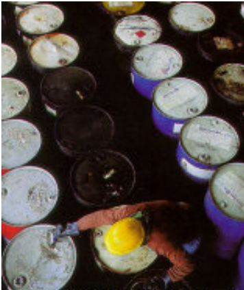
Transport empty drums with all closures in place, with all original hazard markings and labels legible
